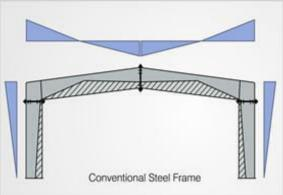
In PEB structure, tapered I-section is provided based on stress distribution along the frame. Multiple trials are preferred to get the optimized steel section for PEB structures. In below diagram, member is designed as per the stress distribution over the span.
